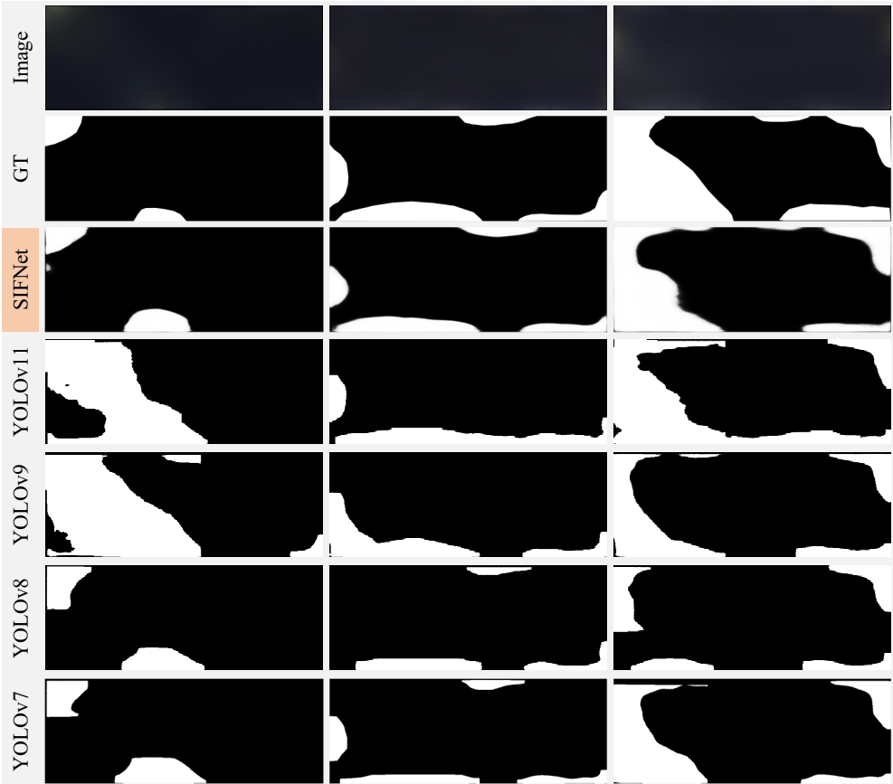
Figure 4. Visual comparison of Mura defect detection results under the black screen scenario.
