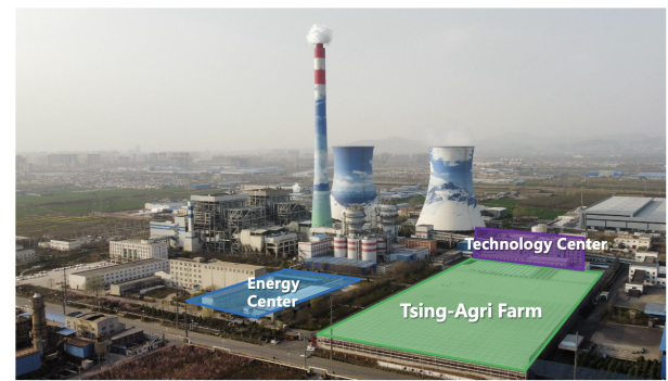
Figure 3. Schematic Layout of the Tsing-Agri Farm Integrated with Mengdian Power Plant.
