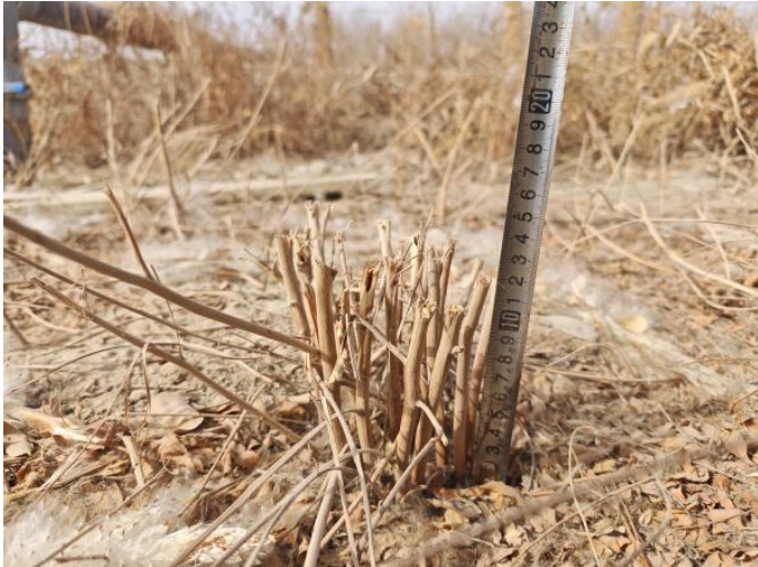
Figure 9. Post-harvest field measurement of stubble height, demonstrating the low-cutting capability of the reciprocating device.
