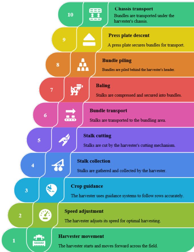
Figure 6. Harvesting workflow of the Apocynum venetum cutting-bundling harvester, from pre-harvest monitoring and crop separation through basal reciprocating cutting, stem folding, vertical obstruction-resistant conveyance, cord-based bundling, crop-plate compaction, and chassis-mounted conveyance of formed bales.
