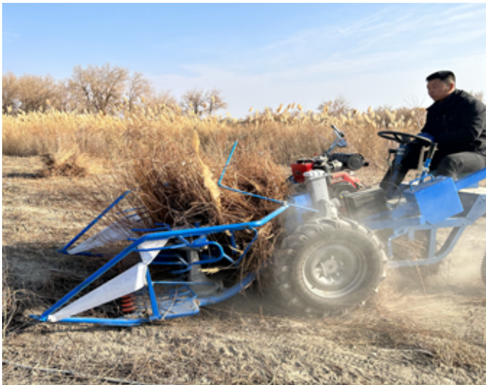
Figure 16. Field prototype of the Apocynum venetum bundling harvester during validation trials in Xinjiang, demonstrating integrated operation under commercial planting conditions with drip-irrigated paired rows and clustered stem stands.
