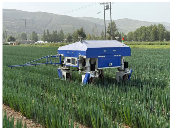
Figure 4. Precision field operation of the targeted variable-rate spraying robot.
