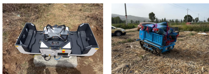
Figure 5. Fully automated UAV inspection and unmanned transport system: (a) UAV dock with UAV; (b) unmanned transport robot.
