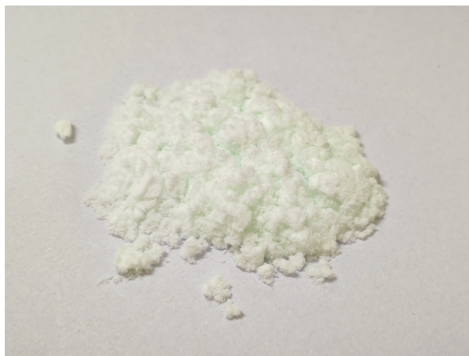
Figure 1. Photograph of the NALF:Cr 3+ phosphor with x = 0.08 .
