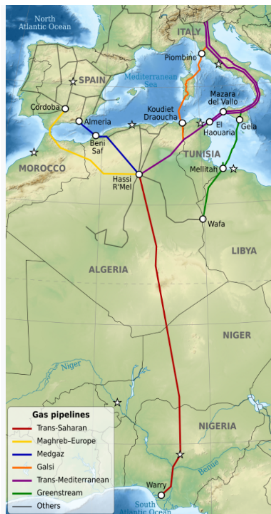
Figure 6. Major gas export pipelines from North and West Africa to Europe. The map illustrates the key operational and planned infrastructures forming the Southern Gas Corridor: (i) The Transmed (Trans-Mediterranean Pipeline) transports Algerian gas via Tunisia to Italy, with a capacity of 33 bcm/year. (ii) The Medgaz Pipeline directly links Algeria (Beni Saf) to Spain (Almería), with a capacity of 10–11 bcm/year. (iii) The Gazoduc Maghreb-Europe (GME) crosses Algeria, Morocco, and the Strait of Gibraltar to supply Spain, with a former capacity of 12–13 bcm/year (currently inactive since 2021). (iv) The proposed Galsi Pipeline would link Algeria to Sardinia and mainland Italy, with a planned capacity of 8 bcm/year. (v) The Trans-Saharan Gas Pipeline (TSGP) , under consideration, would connect Nigeria to Algeria via Niger, enabling up to 30 bcm/year of gas exports to Europe. (vi) The Africa Atlantic Gas Pipeline (AAGP/NMGP) is a planned 5,600 km project from Nigeria to Morocco, intended to supply West African nations and connect to Europe via the GME corridor, with a potential capacity of 30 bcm/year. These infrastructures collectively form a strategic alternative to Russian gas imports, enhancing EU energy security and fostering transcontinental energy cooperation. Source: [67].
