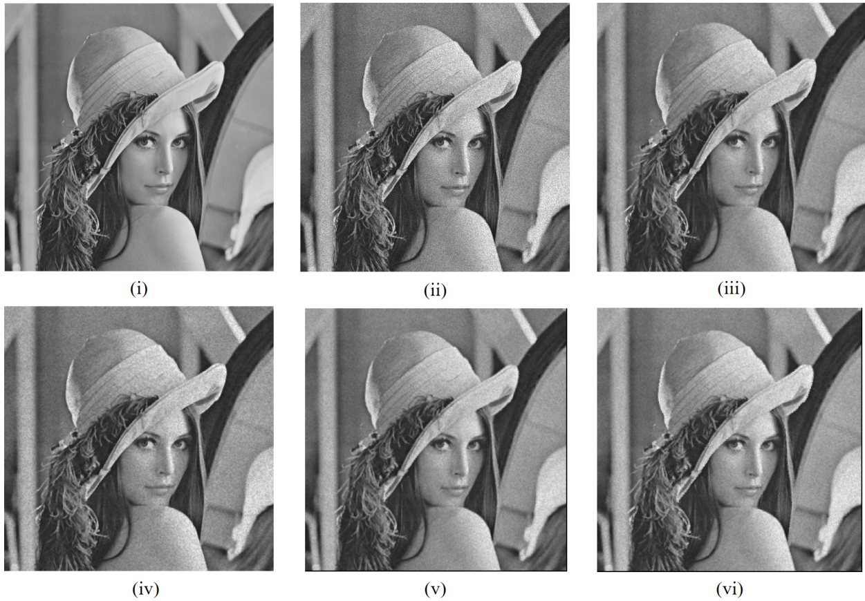
Figure 5. Performance Comparison of Noise Reduction Filters on “Lena” Image: (i) Original image, (ii) Image affected by 10% speckle noise, (iii) Denoised using the wiener filter, (iv) Denoised using the median filter, (v) Denoised using the triangular fuzzy filter, and (vi) Denoised using the proposed fuzzy filter.
