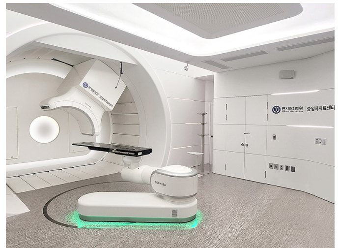
Figure 9. Treatment room with a rotating gantry for carbon-ion hadron therapy (image: Toshiba Energy Systems & Solutions Corporation, 2024; permission to be confirmed).
