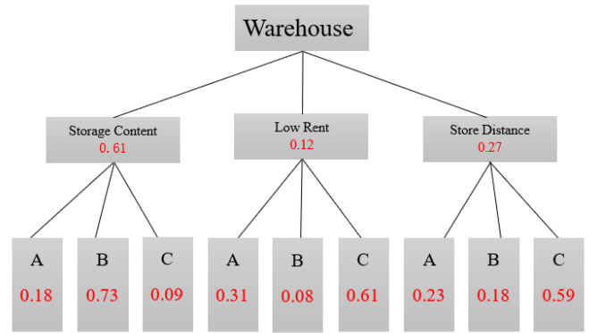
Figure 2. Warehouse location hierarchy diagram.
