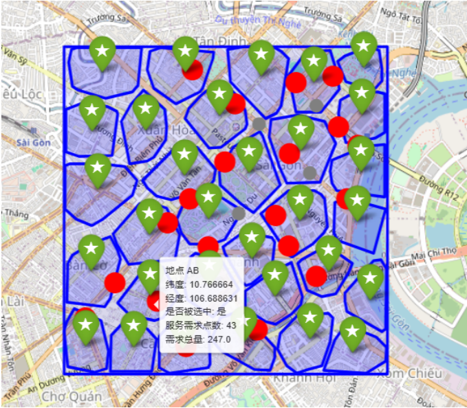
Figure 20. Spatial distribution of 31 optimally located candidate charging stations across District 1 for 2029 under budget constraints, revealing persistent spatial hierarchy with core commercial stations absorbing 58.7% of total district demand despite occupying only 22.6% of geographic area. Northern residential stations (O, G, AE) show emerging demand concentration (+8.4% growth since 2026), signaling gradual residential electrification while commercial cores remain dominant demand generators.
