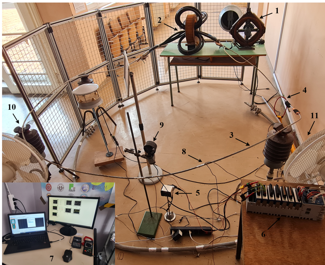
Figure 1. Overview of the experimental setup used for AC resistance and thermal measurements of the investigated ACSR conductor: (1) variable autotransformer, (2) step-down transformer, (3) ACSR conductor, (4) current probe, (5) NI-9215 module, (6) NI cDAQ-9133 data acquisition chassis, (7) laptop with external monitor, (8) temperature sensors, (9) anemometer, (10) support insulator, and (11) fan.
