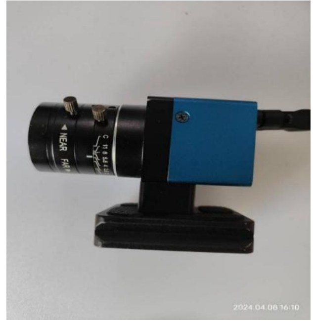
Figure 1. Daheng Mercury II MER-500-7UC-L industrial camera.
