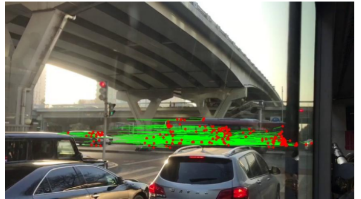
Figure 3. Visualization results of optical flow tracking.
