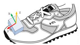
Figure 1. The IMU is fixed on the shoes.
