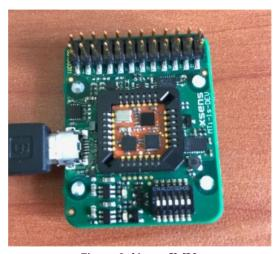
Figure 2. Xsens IMU.
