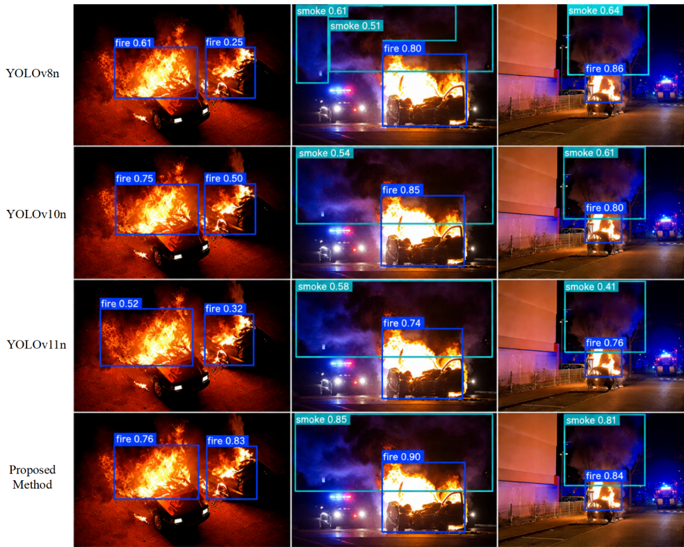
Figure 7. Qualitative comparison of detection results on representative nighttime fire scenes.
