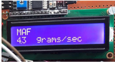
Figure 11. MAF during Test.
