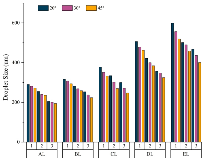
Figure 5. Particle size information of atomization field axial section at different spray angles.
