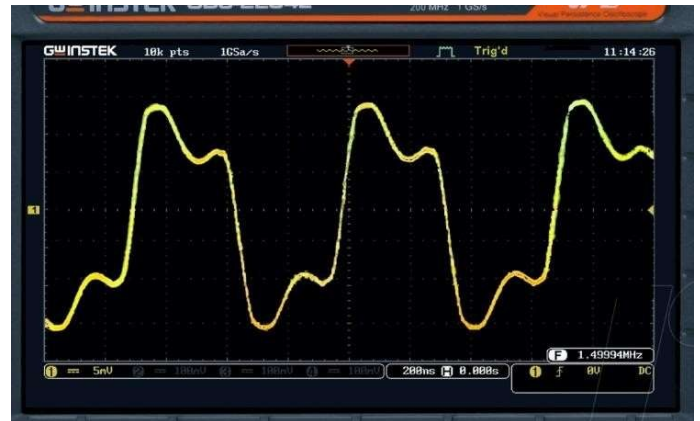
Figure 6. Transformer Output Waveform.
