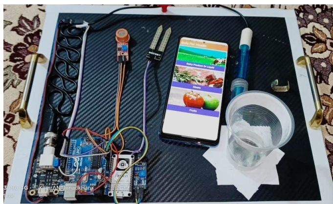
Figure 6. Complete project setup featuring pH, moisture, and ethanol sensors integrated with Arduino UNO and NodeMCU.
