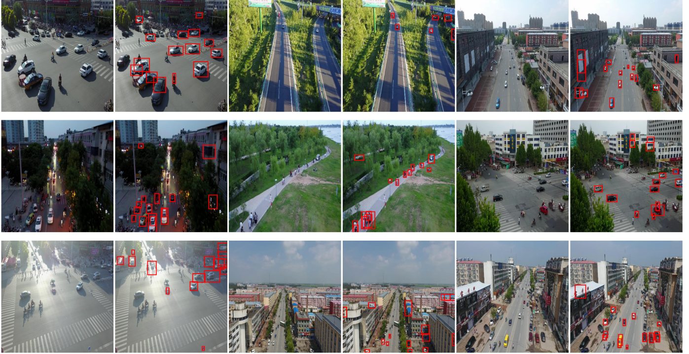
Figure 6. Qualitative detection results of MS-CADNet on VisDrone-DET. Green boxes indicate correct detections of small pedestrians, cyclists, and vehicles.
