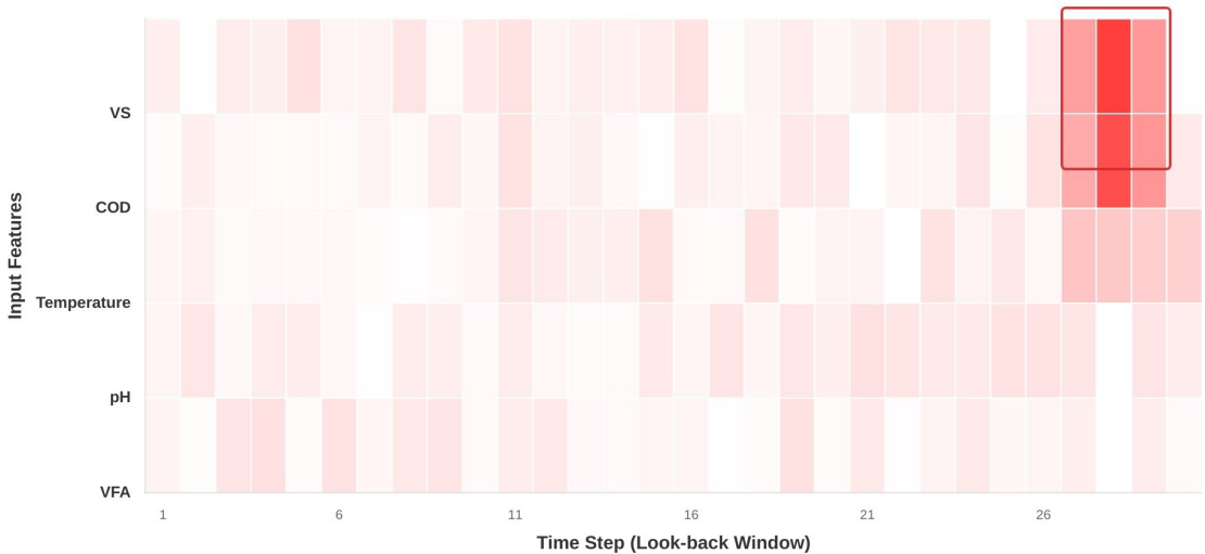
Figure 5. Heatmap of average attention weights ( \alpha_t ) assigned by the model to the top five input features over the 30-step look-back window.
