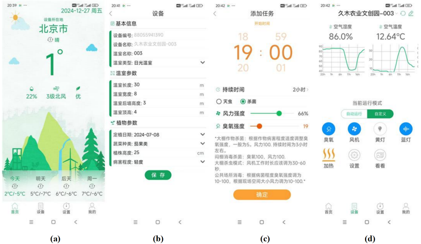
Figure 2. Control interfaces of the mobile phone app for the plant protection device. (a) Login interface, (b) device registration interface, (c) device operation mode interface, and (d) operating device interface.
