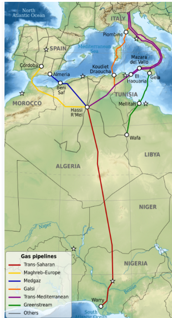
Figure 6. Major gas export pipelines from North and West Africa to Europe. The map illustrates the key operational and planned infrastructures forming the Southern Gas Corridor: (i) The Transmed (Trans-Mediterranean Pipeline) transports Algerian gas via Tunisia to Italy, with a capacity of 33 bcm/year. (ii) The Medgaz Pipeline directly links Algeria (Beni Saf) to Spain (Almería), with a capacity of 10–11 bcm/year. (iii) The Gazoduc Maghreb-Europe (GME) crosses Algeria, Morocco, and the Strait of Gibraltar to supply Spain, with a former capacity of 12–13 bcm/year (currently inactive since 2021). (iv) The proposed Galsi Pipeline would link Algeria to Sardinia and mainland Italy, with a planned capacity of 8 bcm/year. (v) The Trans-Saharan Gas Pipeline (TSGP) , under consideration, would connect Nigeria to Algeria via Niger, enabling up to 30 bcm/year of gas exports to Europe. (vi) The Africa Atlantic Gas Pipeline (AAGP/NMGP) is a planned 5,600 km project from Nigeria to Morocco, intended to supply West African nations and connect to Europe via the GME corridor, with a potential capacity of 30 bcm/year. These infrastructures collectively form a strategic alternative to Russian gas imports, enhancing EU energy security and fostering transcontinental energy cooperation. Source: [67].
