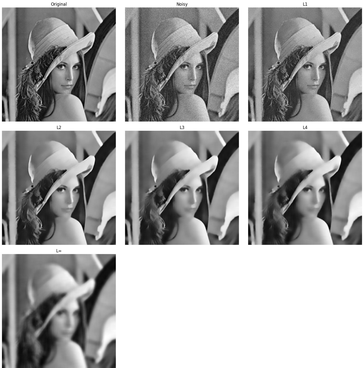
Figure 3. Visual comparison of denoised images under various L_p norms. Note over-smoothing and edge loss for p = \infty , and robustness of p = 2 .
