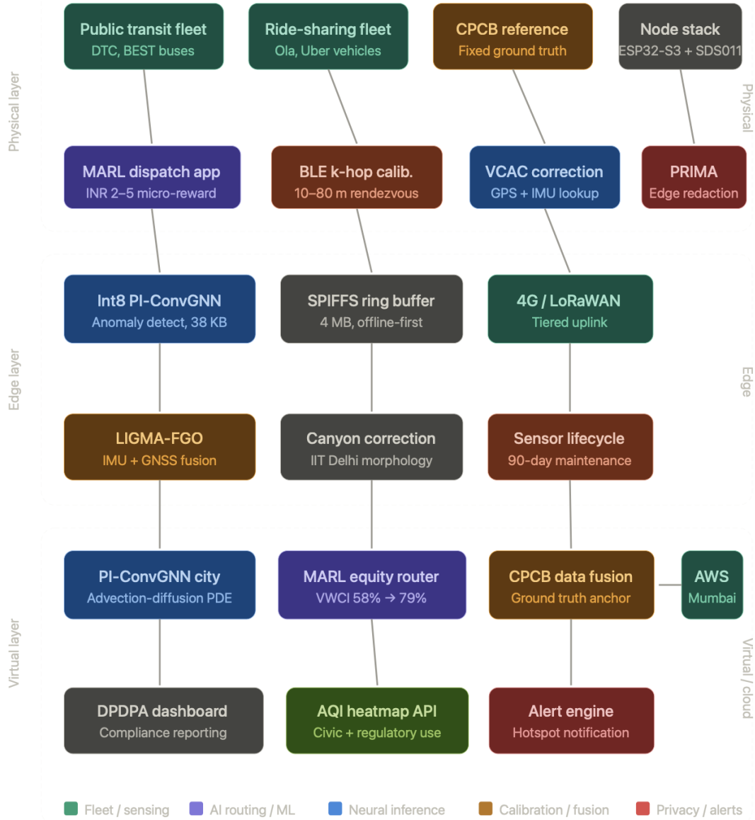
Figure 1. EcoPulse-India three-layer AIoT architecture. The physical layer integrates public-transit and ride-sharing fleets, CPCB reference stations, and embedded sensing nodes. The edge layer provides local calibration, privacy-preserving preprocessing, lightweight neural inference, positioning correction, data buffering and communication, and sensor lifecycle management. The virtual/cloud layer performs city-scale PI-ConvGNN inference, MARL-based coverage optimisation, CPCB data fusion, compliance reporting, AQI visualisation, and hotspot alerting.
