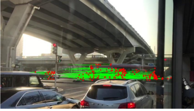
Figure 3. Visualization results of optical flow tracking.
