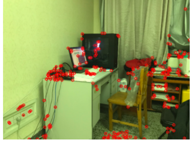
Figure 4. Image of extracting feature points without mask.
