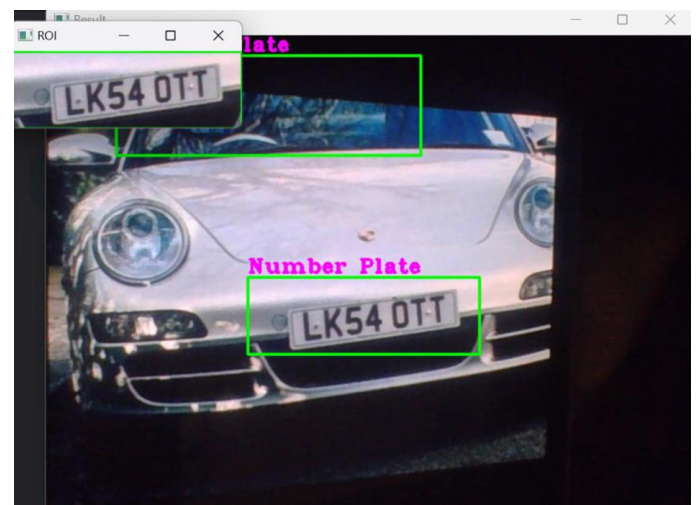
Figure 5. Sample output of license plate recognition showing detected plate and recognized characters.
